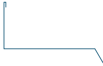
Wall to Roof Flashing 2
