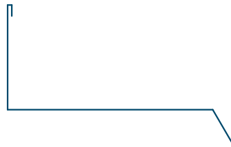
Wall to Roof Flashing 2
