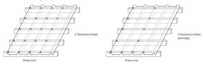
Can be installed over plastic cavibat battens.
