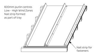
Can be installed as a wall cladding with a substrate over vented cavity battens.
