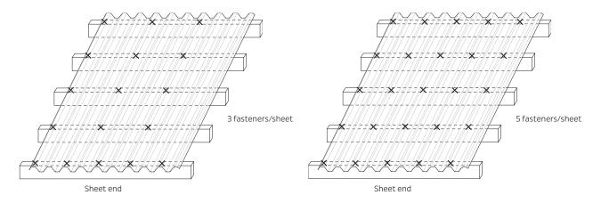
Can be installed over plastic cavibat battens.
