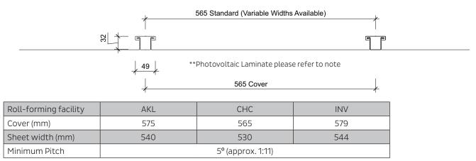
Note for Copper and Zinc reduce widths by 10mm
